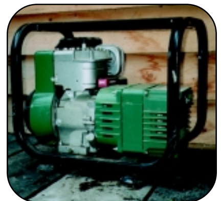
A gasoline-powered generator will allow you to operate your well pump during a power outage.
